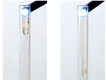
Left: Ivocerin-containing monomer showing high photoreactivity Right: Camphorquinone-containing monomer showing low photoreactivity
